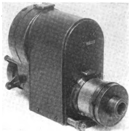
Eisemann impulse starter and coupling mounted on magneto
